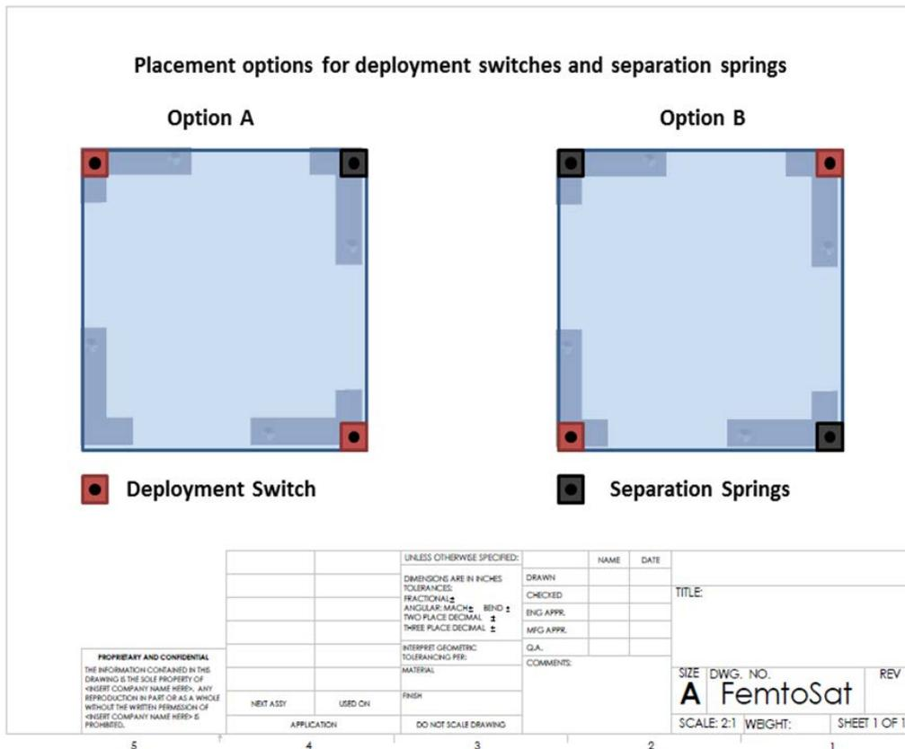
**Figure 5: Deployment Switches and Separation Spring Locations**
