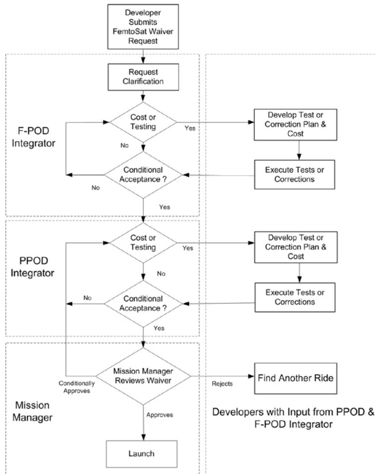
**Figure 2: SunCube FemtoSat Standard Deviation Wavier Process Flow Diagram**
