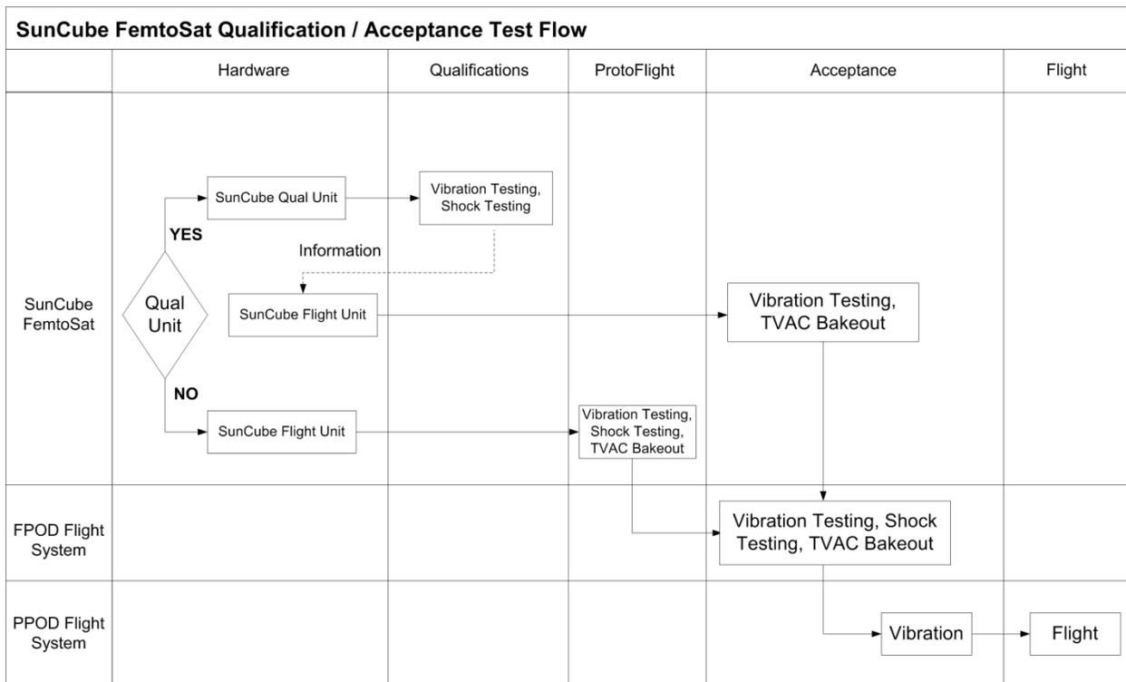
**Figure 7: SunCube FemtoSat General Testing Flow Diagram**
