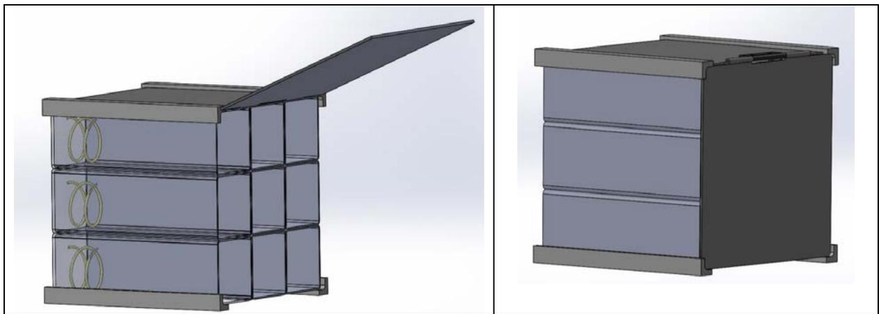
**Figure 3: FemtoSat deployer single and multiple units**
